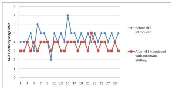
**Figure 07: Daily grid electricity usage before HES introduced and after introduced with automatic shifting**
