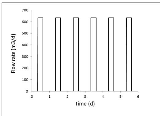
**Figure 3: Input flow pattern (semi continuous feeding) to reactor**
