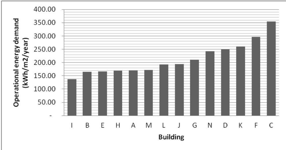
Figure3: Operational energy demand of high rise office buildings in Sri Lanka
