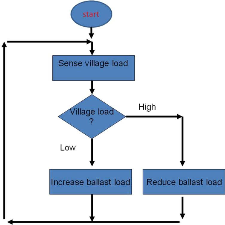
a) Feedback control loop of electric load controller
