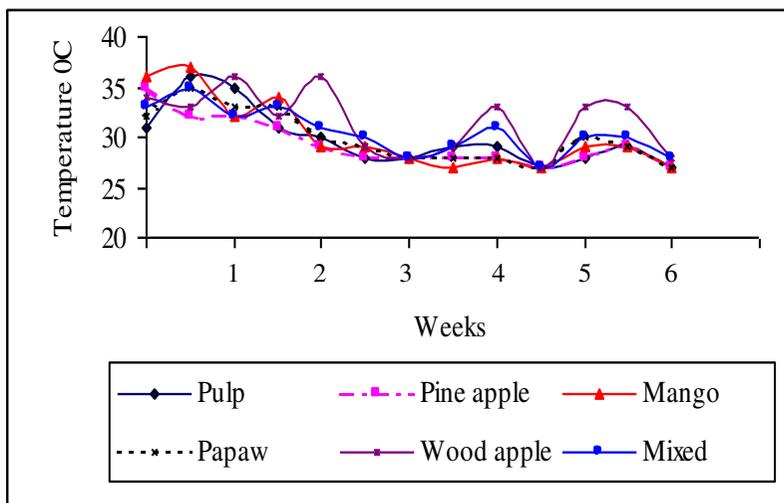
**Figure 05: Temperature Variation with Time in fruit waste Systems**
