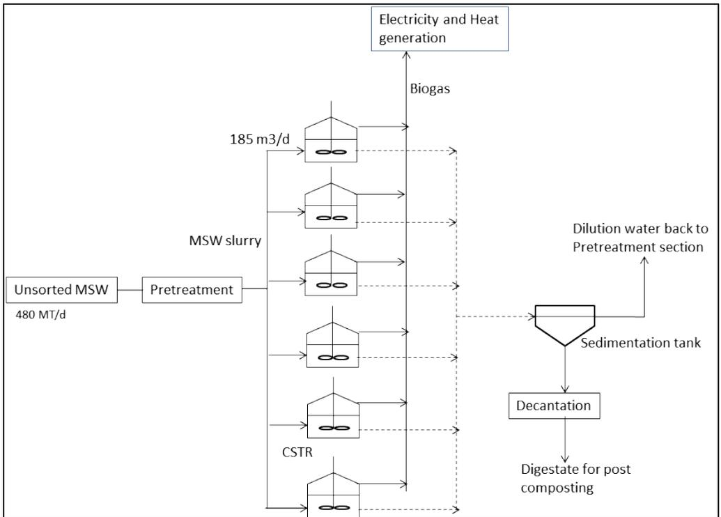
Figure 1: Schematic diagram of simplified large scale anaerobic digestion plant
