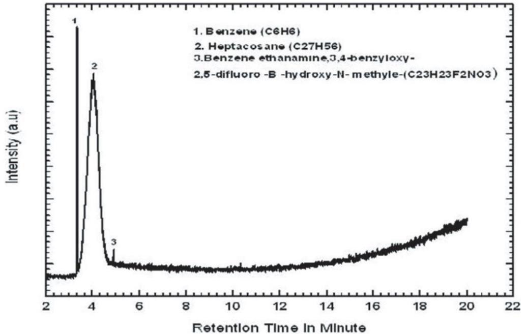
Figure 2: GC/MS chromatogram for fuel produced using PET[4]
