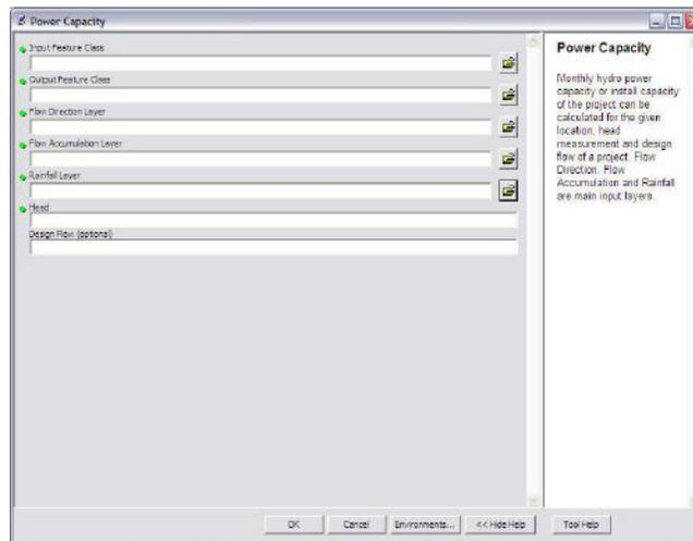
Figure 8: Illustration of Power capacity tool
