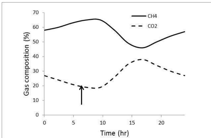
**Figure 6: Simulated biogas composition variation following daily feeding.**
