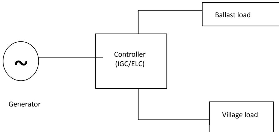
**Figure 1: Ballast and user load connection**
