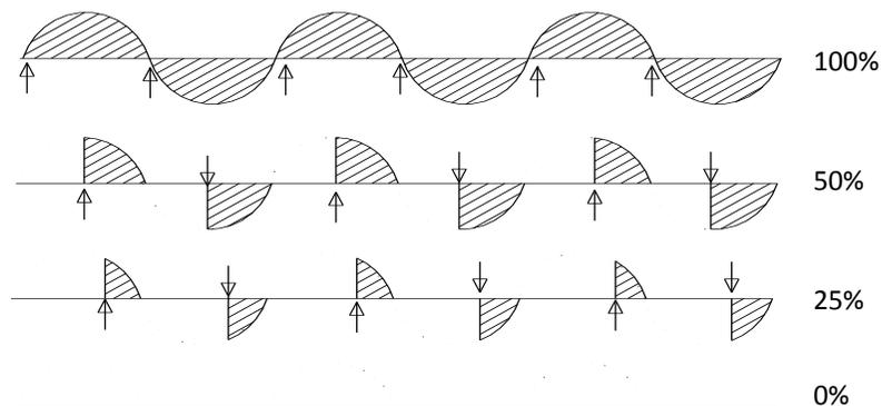
**Figure 4: Wave form of a TRIAC controlled AC power system at different load percentages**
