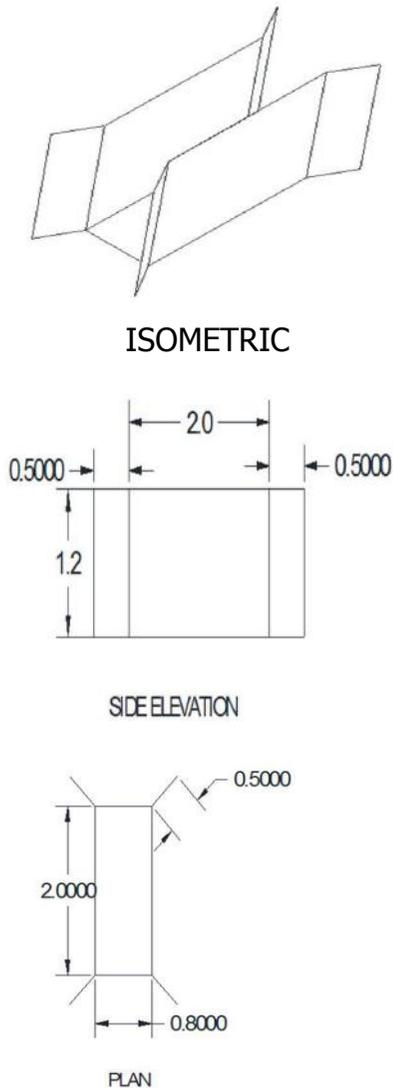
**Figure 3: Drawings of the model manipulator**
