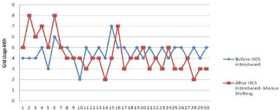
**Figure 06: Daily grid electricity usage before HES introduced and after introduced with manual shifting**
