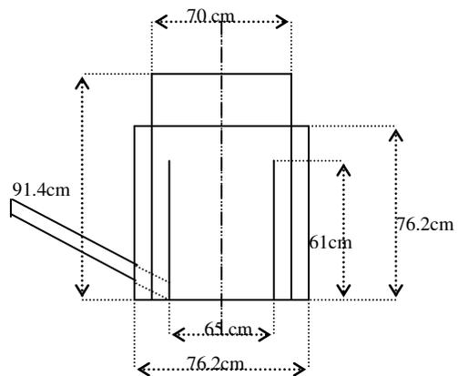
**Figure 01: Schematic diagram for preliminary stage digester**
