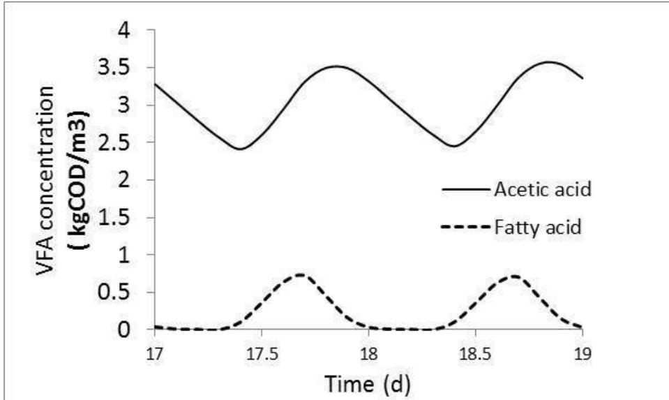
Figure 9: Volatile fatty acids variation in the liquid phase.
