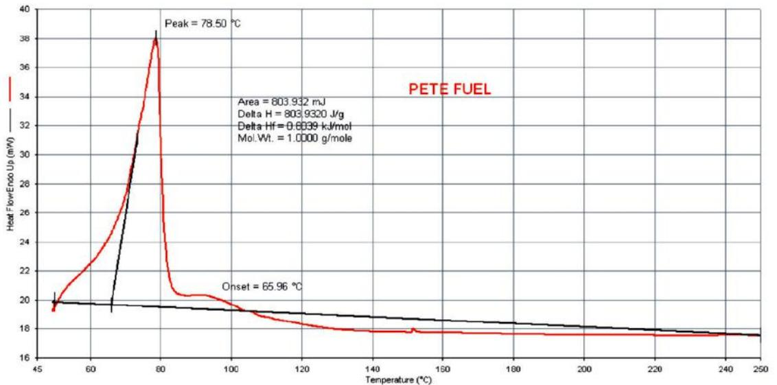
Figure 3: Differential Scanning Calorimeter DSC curve for liquid fuel produced using PET[4]
