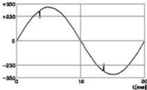
**Figure 7: Wave form distortion when ballast turns ON in peak range of wave (source [5])**
