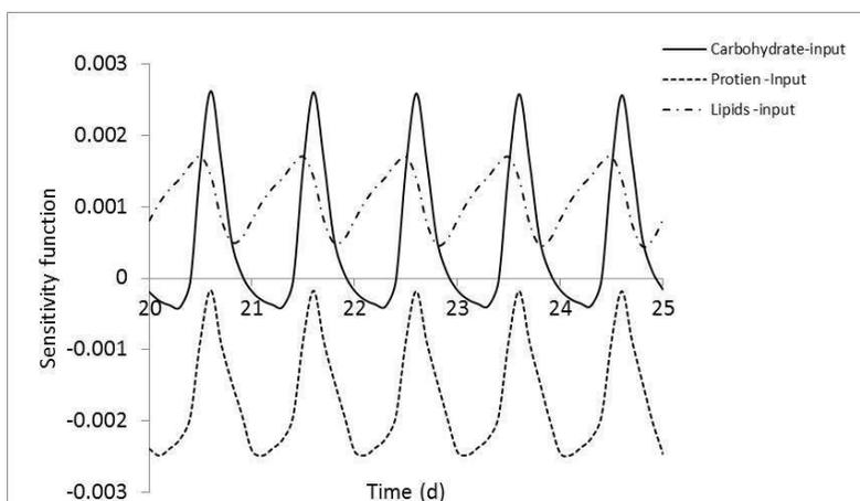
**Figure 5: Sensitivity of input constituents towards CO<sub>2</sub> composition of biogas**
