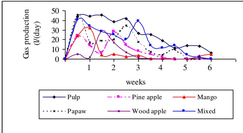
**Figure 03: Daily biogas production rate with time**
