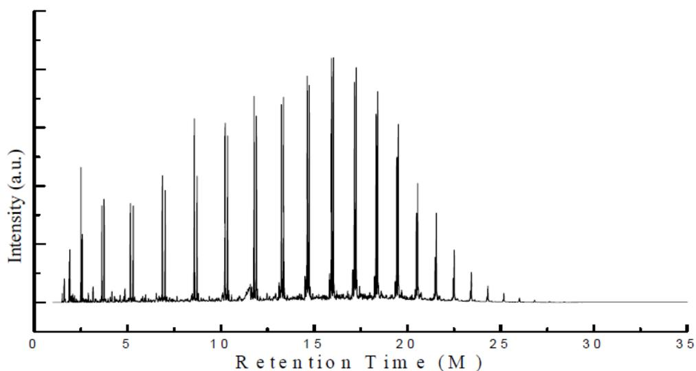
**Figure 4: The GC/MS chromatogram of the fuel mixture obtained through thermal degradation of PET and LDPE mixture[11]**
