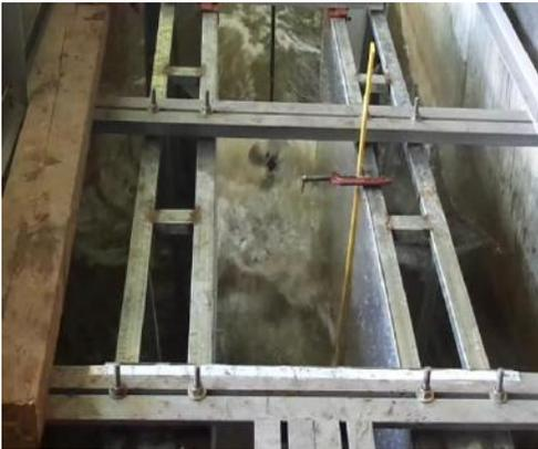
**Figure 5: Turbine placed in the tunnel end**
