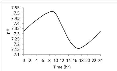
**Figure 8: pH variation inside bulk liquid after feeding**
