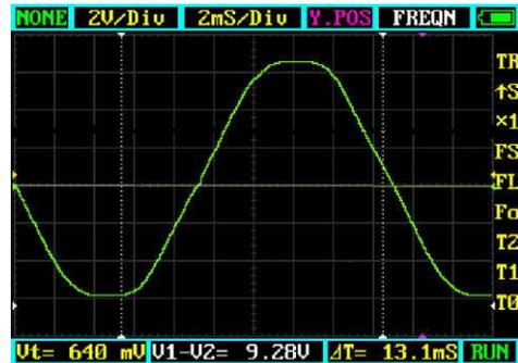
**Figure 12: Wave form of a Multiple, loads zero crossin point switching controller**
