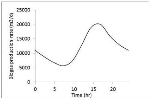
**Figure 7: Biogas production rate following feeding**
