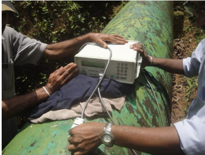
Figure 16: Flow measurement during performance evaluation of a small hydro plant
