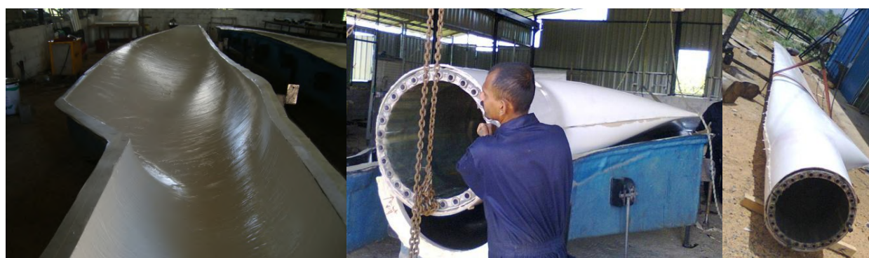
Figure 9: Local manufacture of wind turbine blades
