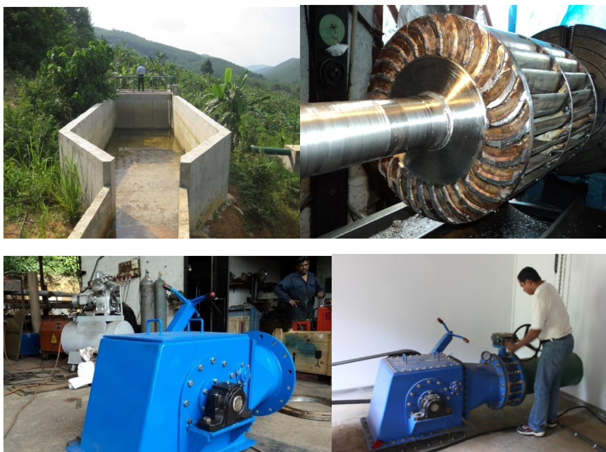
Figure 10: Channel and the locally manufactured hydro turbine
