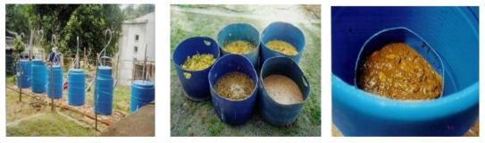
Figure 2a: Batch fed barreled digesters Figure 2b: Substrate were mixed with cow dung & water
