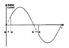
Phase angle controller Figure 8: Phase angle control of TRIAC (source [4])
