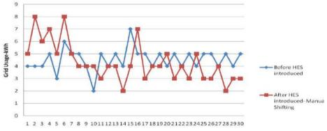
Figure 06: Daily grid electricity usage before HES introduced and after introduced with manual shifting
