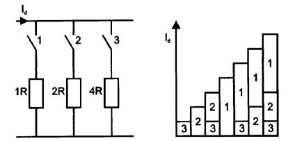
Fig. 6 - Binary Weighted load controller (source [4])
