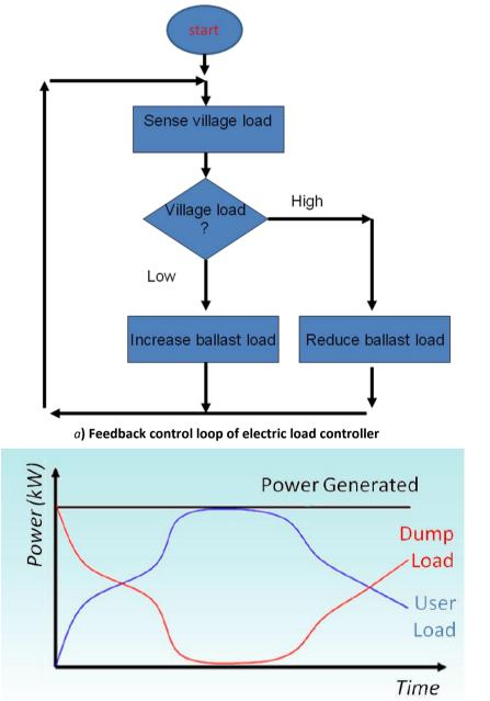
b) Constant power generation and consumption while consumer load varies randomly (Source [5]) Figure 3: Electric load controlling process
