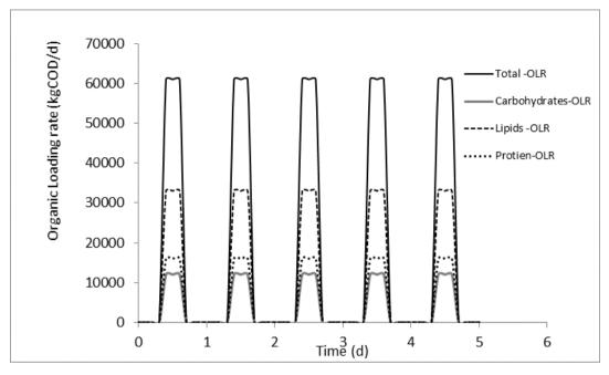
Figure 4: Input organic loading rates (OLR) to ADM1 model.
