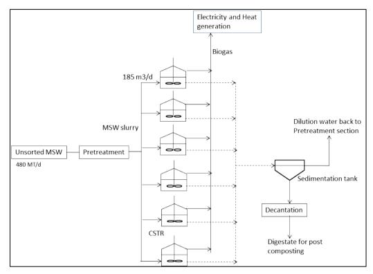
Figure 1: Schematic diagram of simplified large scale anaerobic digestion plant
