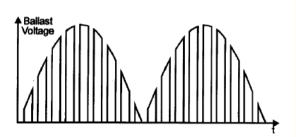
time, thus the process is called Mark-Space ratio. Modern electronic literature refers to this process as Pulse Width Modulation (PWM) [6]. The ballast and consumer wave forms of this control are shown in Fig. 10.
