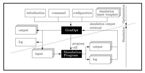
Figure 1: Coupling of GenOpt and a whole building simulation program [8]
