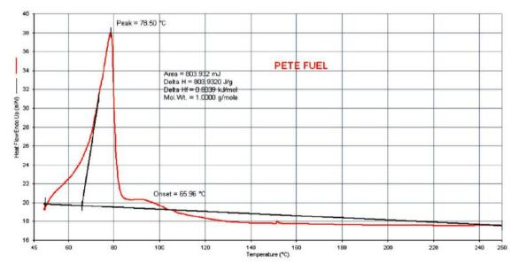
Figure 3: Differential Scanning Calorimeter DSC curve for liquid fuel produced using PET[4]
