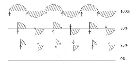
Figure 4: Wave form of a TRIAC controlled AC power system at different load percentages
