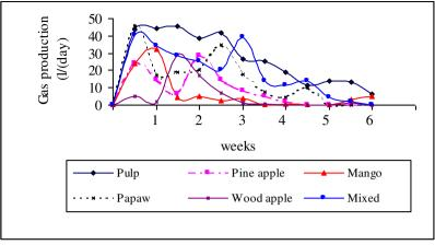
Figure 03: Daily biogas production rate with time
