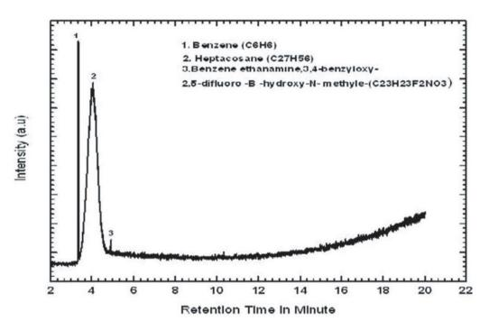
Figure 2: GC/MS chromatogram for fuel produced using PET[4]
