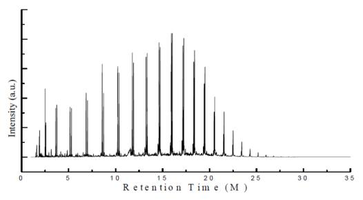
Figure 4: The GC/MS chromatogram of the fuel mixture obtained through thermal degradation of PET and LDPE mixture[11]
