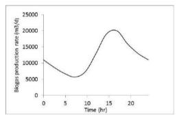
Figure 7: Biogas production rate following feeding
